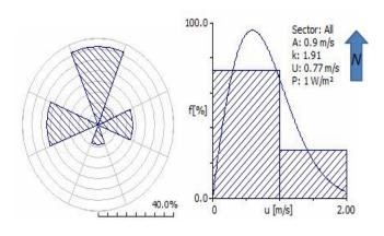
Figure 6.3 Wind Char. at Environmental Lab. (Mine Site) Observed Wind Climate 4/3/2011 to 10/5/2011
