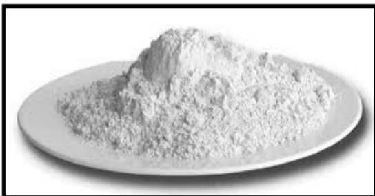
Fig 1 : Appearance of Slag
