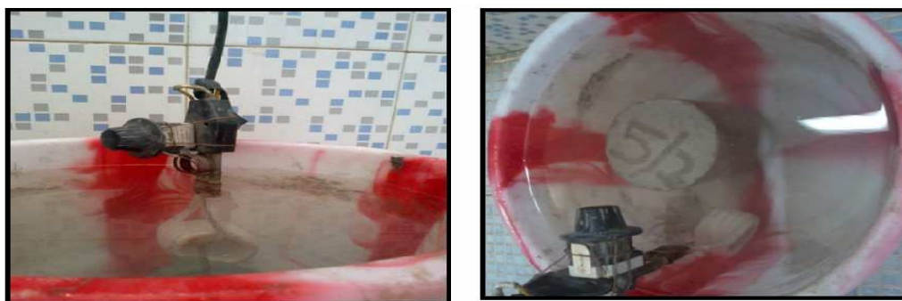
Fig 2 : Specimens under thermal curing
