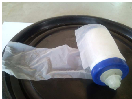
Fig.1 Nylon cloth wrapped around a yarn cartridge
