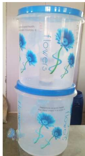
Fig. 2 Domestic defluoridation unit (11 lit.) capacity with single yarn cartridge
