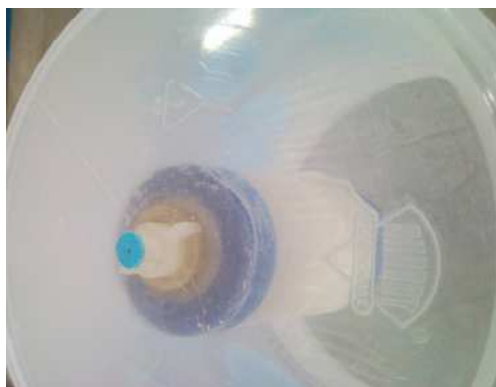
Fig. 3 Flow rate control plastic pin hole fitted at the outlet of the yarn cartridge
