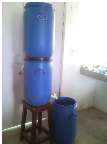
Fig. 4 Intermediate level defluoridation unit (50 lit.) capacity with double yarn cartridge
