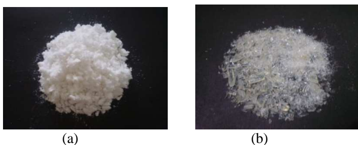
Figure 1. \alpha -cellulose (a) and nanocrystalline cellulose (b) of sugar palm bunches
