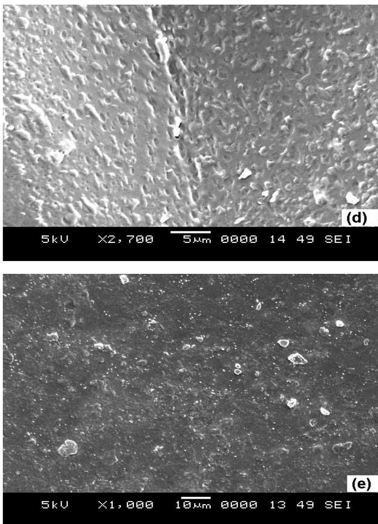
**Figure 6a-6e.** SEM images of films consisting of (a) pure PSSA, (b) 80/20, (c) 50/50, (d) 20/80 and (e) pure
