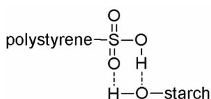
**Figure 3. Schematic interactions between PSSA/starch polymers with hydrogen bonding.**
