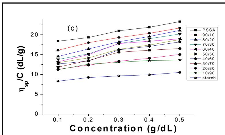
Figure 1. Reduced viscosity versus concentration of PSSA/starch blends at (a) 30 °C (b) 40 °C (c) 50 °C
