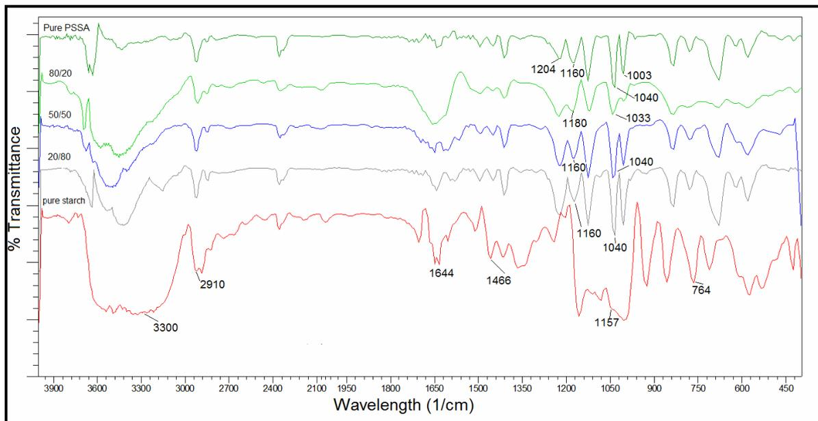
**Figure 4. FTIR spectra of films consisting of pure components and different PSSA/starch blend ratios.**
