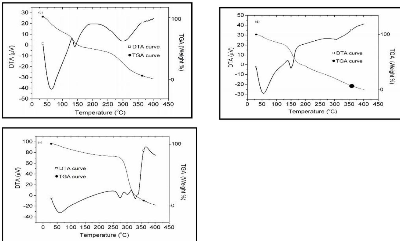
**Figure 5a-5e.** TGA and DTA traces obtained by heating samples from 25 °C to 400 °C at a heating rate of 10 °C/min under nitrogen atmosphere for (a) pure PSSA, (b) 80/20, (c) 50/50, (d) 20/80 and (e) pure starch.
