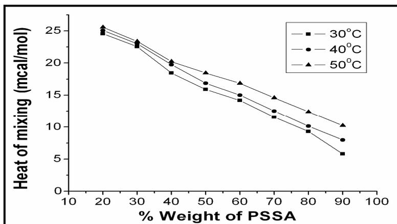
**Figure 2.** Heat of mixing of PSSA/starch blends at different temperatures.
