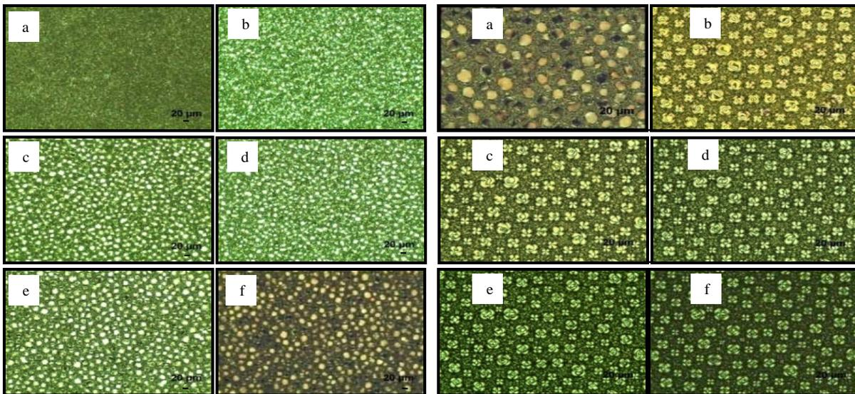
**Figure 1:** Effect of dye concentration (a) 0%, (b) 0.007%, (c) 0.015%, (d) 0.0625%, (e) 0.25%, (f) 1 % on droplet morphology of GHPDLC films.
