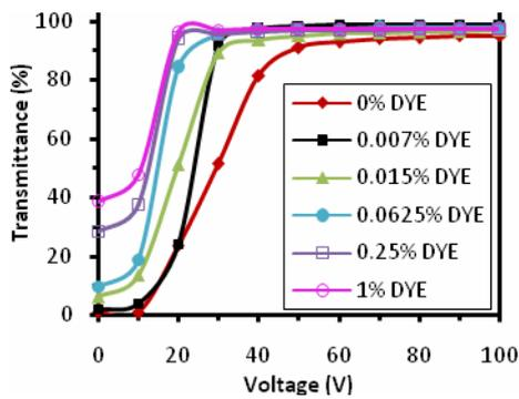
**Figure 3:** Transmittance vs voltage curves of GHPDLC films with various dye concentration at 200 Hz and 25 °C.
