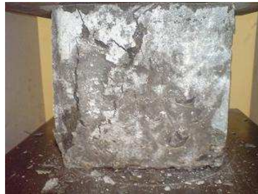
Fig. 6 Crushed state of cube
