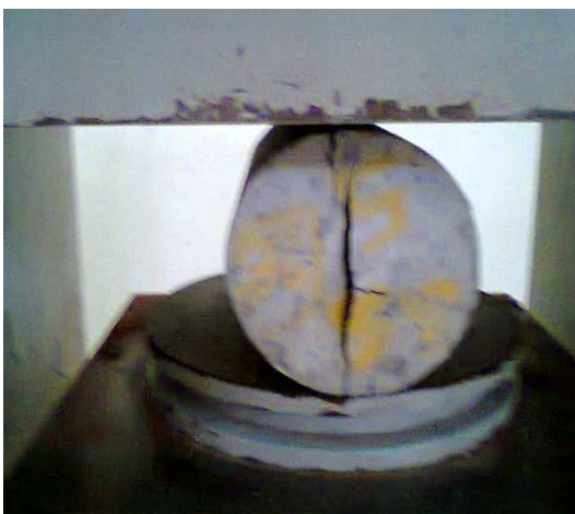
Fig.7 State of cylinder after applying tensile load
