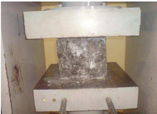
Fig.5 Cube being tested
