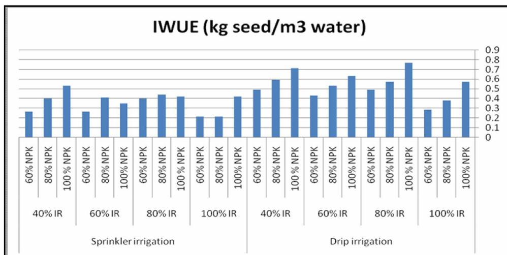
**Fig (5) Effect of interaction between irrigation systems, irrigation water deficit and fertigation rates on irrigation water use efficiency of groundnut seed**
