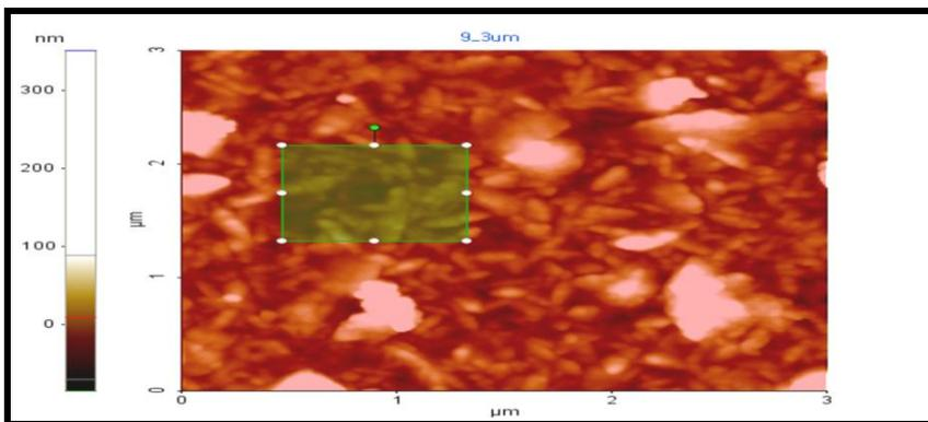
Figure. 4 AFM micrograph of a typical undoped ZnO at 330°C
