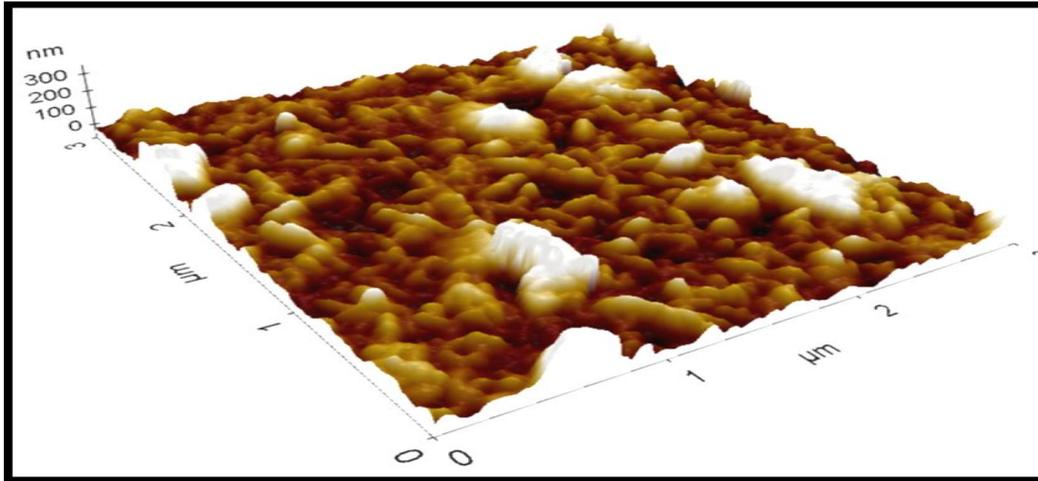
Fig. 8 (3D) Topography for a typical 220°C substrate temperature
