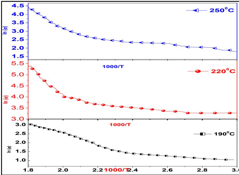
Fig.10 Variation of  $\ln(\sigma)$  Vs  $1000/T$  with substrate temperature
