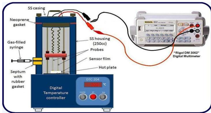
Fig. 1 Schematic diagram of the Gas sensor unit
