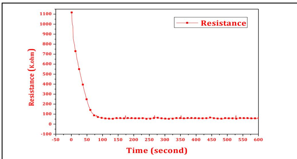
Fig.11 Stabilization curve for ZnO thin film at 300°C operating temperature.
