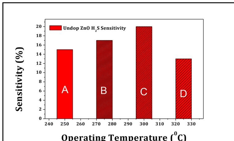
Fig.14 H<sub>2</sub>S gas Sensitivity of ZnO thin film as a function of operating temperature
