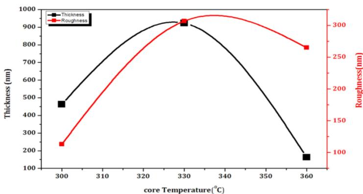
Fig. 5 Variation thickness and roughness of ZnO thin film with core
