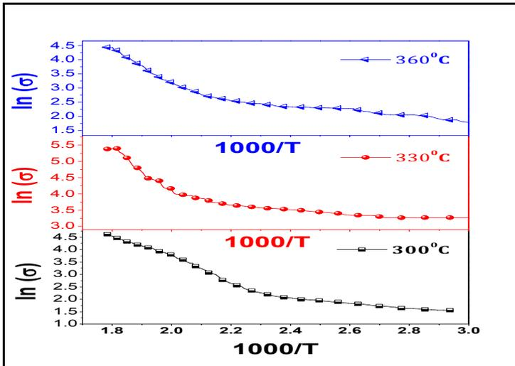
Fig.6 Variation of  $\ln(\sigma)$  with  $(1000/T)$  for ZnO thin film.
