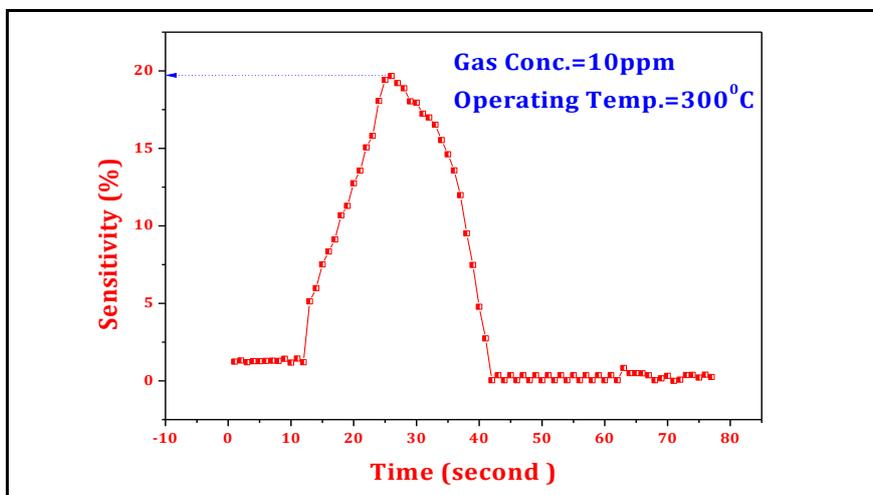
Fig.13 Typical H<sub>2</sub>S gas Sensitivity at 300°C operating temperature for ZnO thin film.
