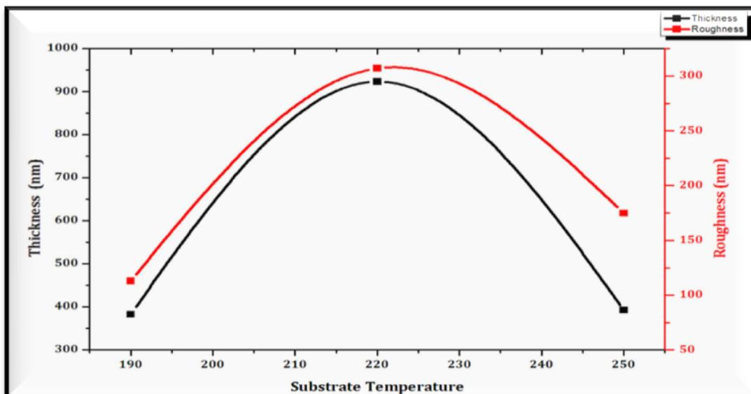
Fig. 9 Variation of Thickness and Roughness with substrate temperature
