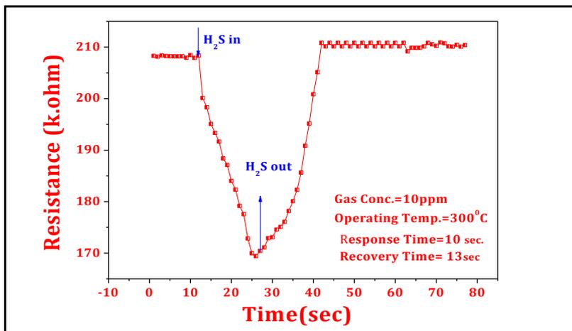
Fig.12 H<sub>2</sub>S gas response of ZnO thin films for 300°C operating temperature.
