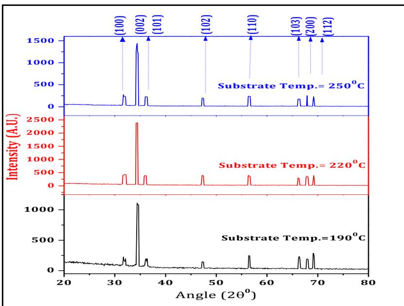
Fig.7 XRD patterns of ZnO thin films with substrate temperature variation
