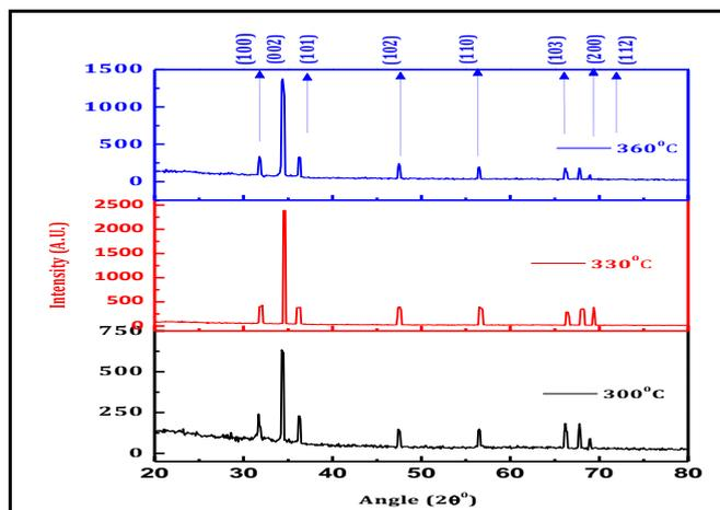
Fig. 2 XRD patterns for core temperature variation of ZnO thin films
