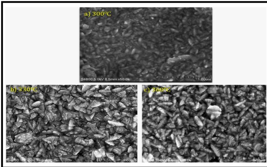
Fig. 3 Plain view FESEM micrographs for ZnO films prepared at various core temperatures
