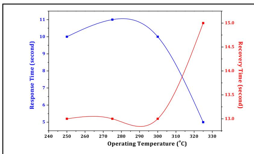
Fig.15 Transient response of H<sub>2</sub>S gas w. r. t. operating temperature.
