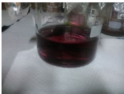
Fig 2.1 Pale pink coloured colloidal gold after citrate reduction
