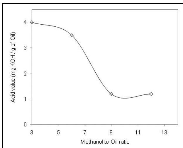
**Figure 3 Effect of Methanol to Oil ratio on transesterification of algae oil**
