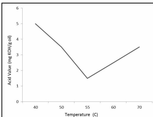
**Figure 2 Effect of Temperature on transesterification of algae oil**
