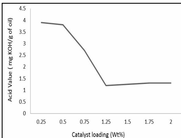
**Figure 4 Effect of Catalyst loading on transesterification of algae oil**
