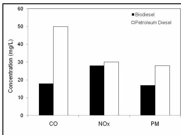
**Figure 5 Comparative analyses of Emissions**
