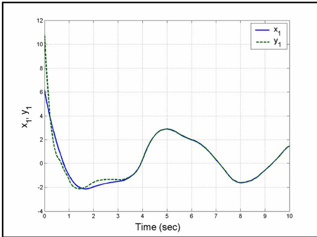
Figure 4. Hybrid chaos synchronization of the states  $x_1$  and  $y_1$
