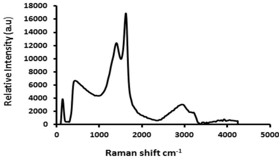
Figure 4. Raman spectra of the synthesized CNTs from IKDPS
