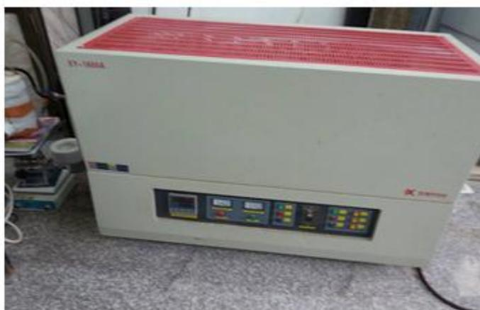
Figure 3. Image of tube furnace that was used in synthesis of CNTs from IKDPS
