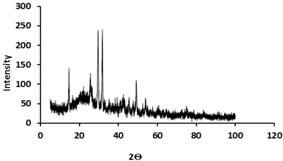
Figure 8. XRD patterns for synthesized CNTs derived from IKDPS
