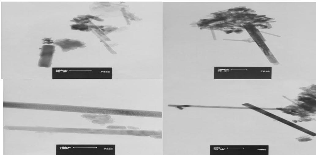
Figure 6. TEM images of synthesized CNTs grown by CVD methods at 750 °C
