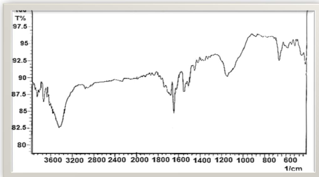
Figure 11. FTIR spectra for the synthesized CNTs from IKDPs
