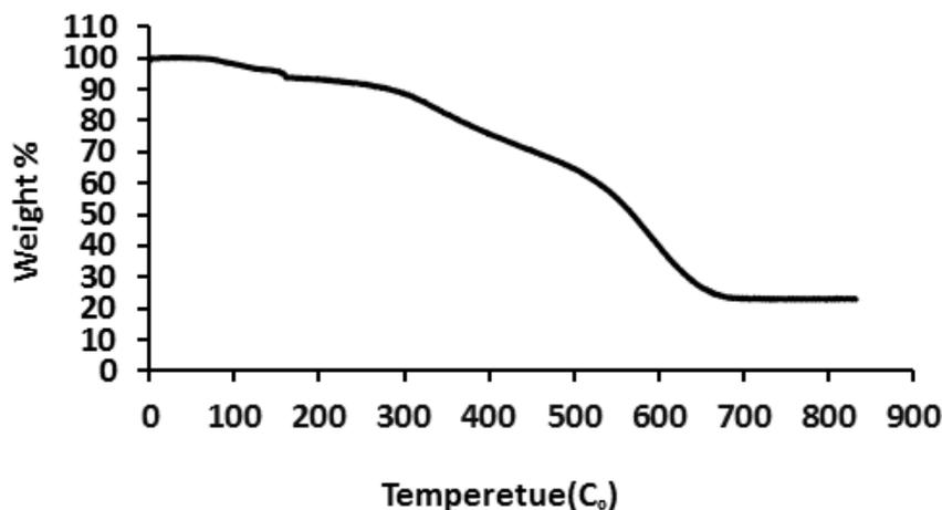
Figure 9. Schematic diagram of TGA graph for the synthesized CNTs.
