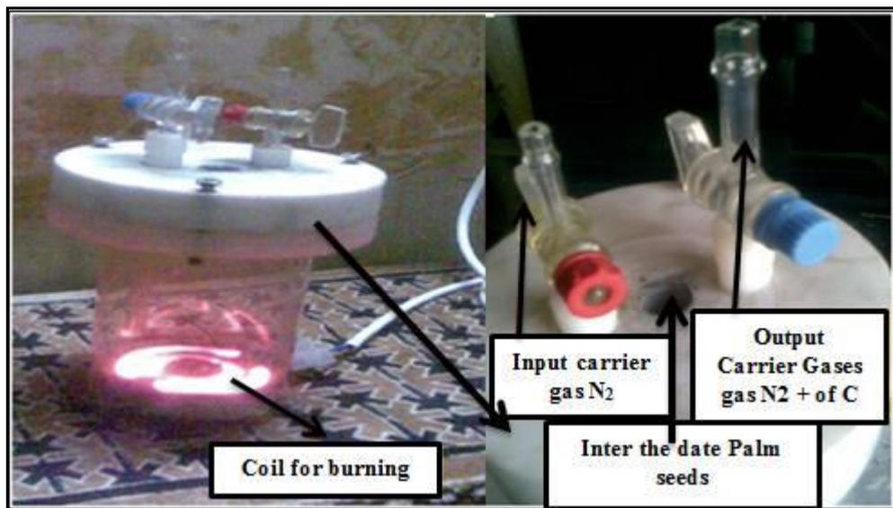
Figure 2. Image description of the used burning reactor that was used in synthesis of CNTs
