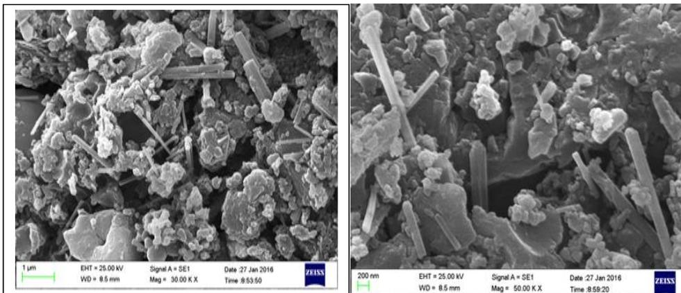
Figure 5. SEM images for the synthesized CNTs from IKDPS
