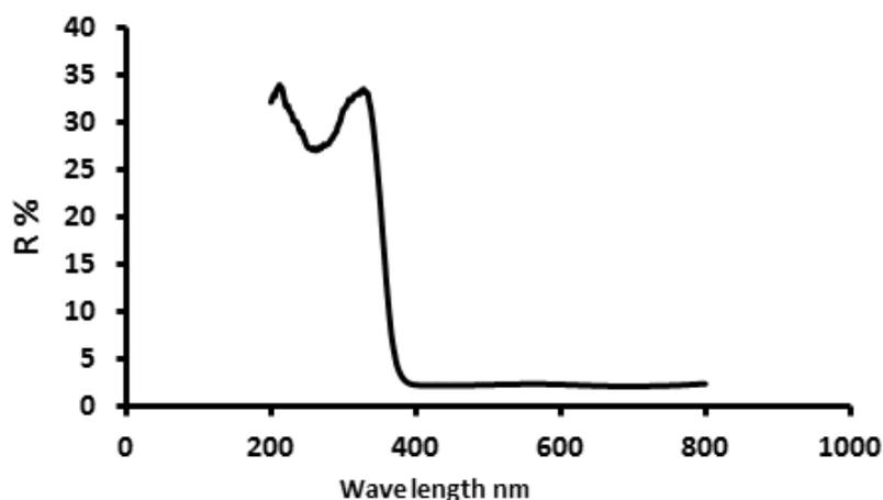
Figure 10. UV- visible reflectance spectrum for synthesized CNTs
