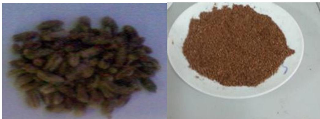
**Figure 1. Image of Iraqi kentar date palm seeds that were used as raw materials for CNTs synthesis**
