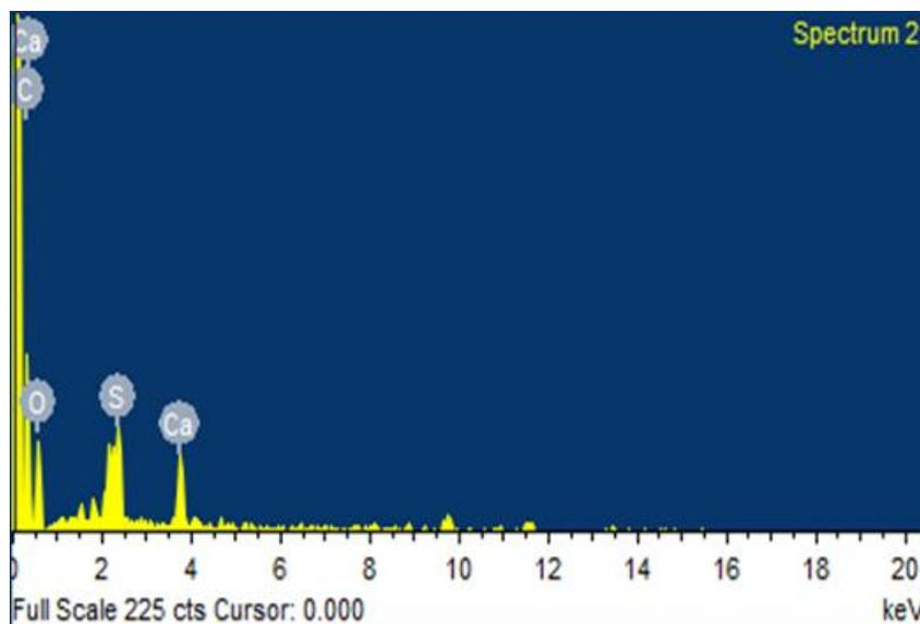
Figure 7. EDX for Synthesized CNTs from IKDPS
