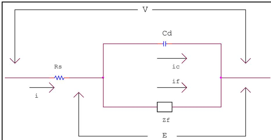
**Fig 1. Equivalent electrical circuit representing the electrochemical cell**
