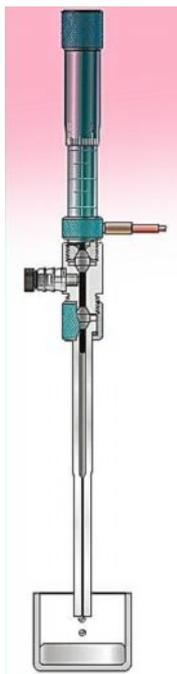
**Fig 3: Schematic of HMDE**
