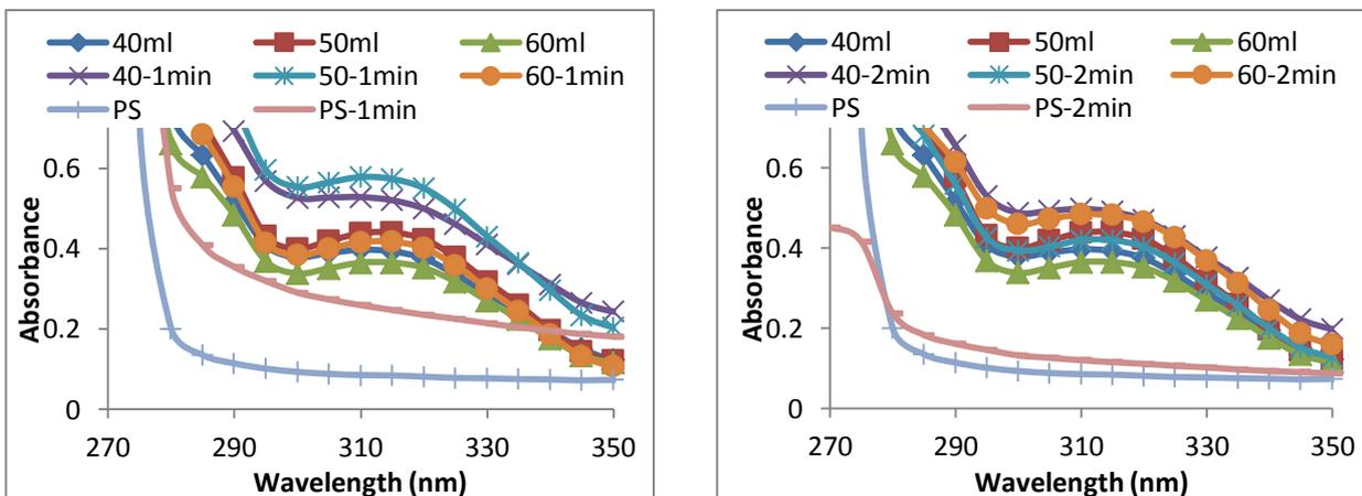
**Figure (3) Absorption spectrum for pure PS and Coumarin doped PS films before and after irradiated**
