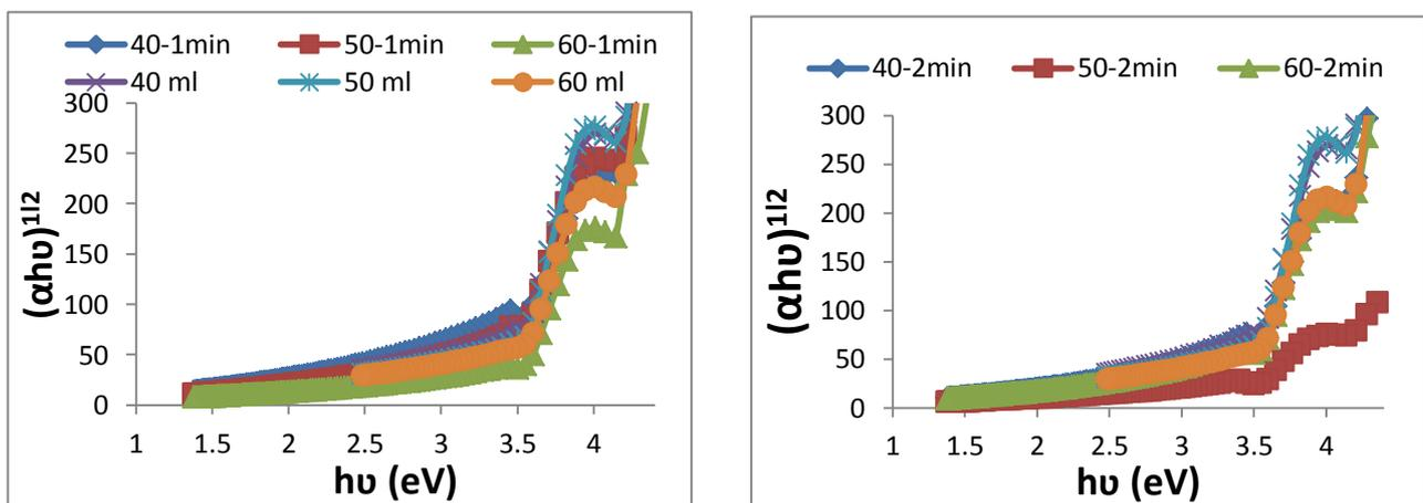
**Figure (7) Energy gap for Coumarin doped PS films before and after irradiated**
