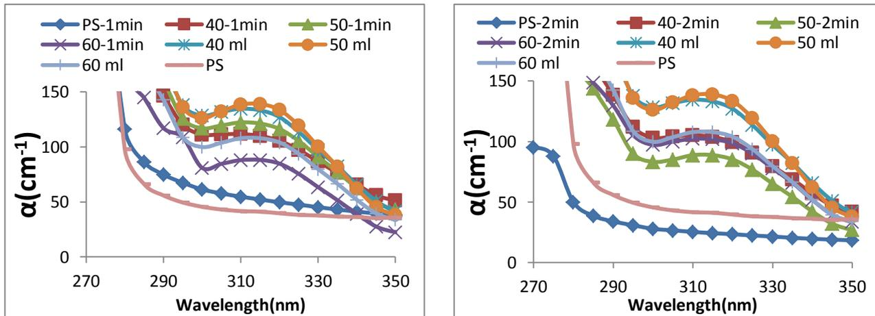
**Figure (6) Absorption Coefficient spectrum for pure PS and Coumarin doped PS films before and after irradiated.**
