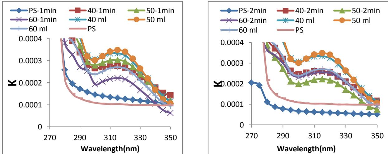
Figure (9) Extinction Coefficient for pure PS and Coumarin doped PS films before and after irradiated
