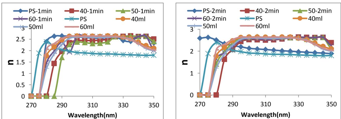
**Figure (8) Refractive Index for pure PS and Coumarin doped PS films before and after irradiated.**
