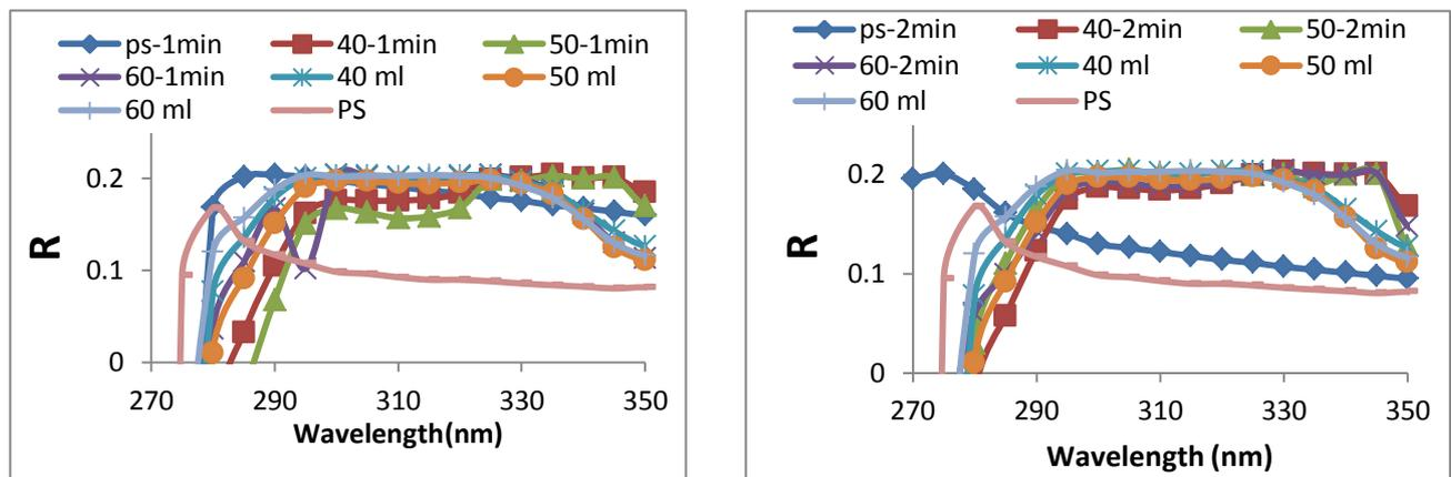
Figure (5) Reflection spectrum for pure PS and Coumarin doped PS films before and after irradiated
