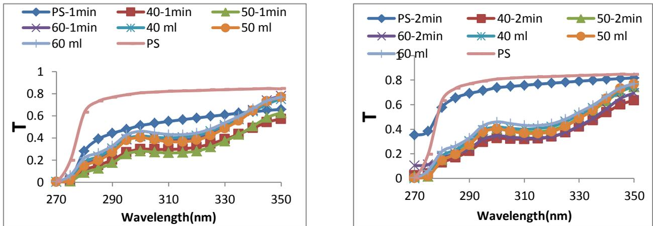
Figure (4) Transmission spectrum for pure PS and Coumarin doped PS films before and after irradiated
