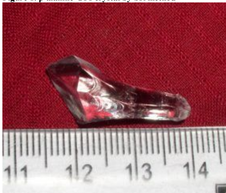
Figure 1. \beta -alanine-GPI crystal by SR method
