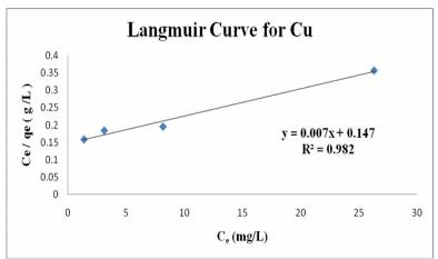
Fig.5 Langmuir adsorption isotherm for Cu by Spirulina sp. (q<sub>max</sub>= 142.85 mg/g, b= 0.047L/mg).
