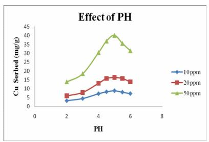
Fig.1 Effect of pH on biosorption of Cu by Sprulina sp.(biomass dose=0.1 g, initial Cu ion concentration = 10, 20 and 50 mg  $\Gamma^{-1}$ ; temperature = 25 °C; agitation speed = 120 rpm; contact time = 120 min).
