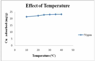
Fig.4 Effect of Temperature on biosorption of Cu by Sprulina sp.(biomass dose=0.1 g, pH=5, initial Cu ion concentration = 50 mg  $\Gamma^{-1}$ ; temperature = 25 °C; agitation speed = 120 rpm; contact time = 120 min).
