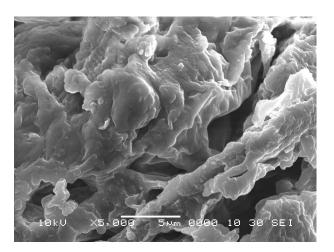
Fig.11 Scanning electron microscopy (SEM) micrographs of the Sprulina sp. after biosorption of Cu.
