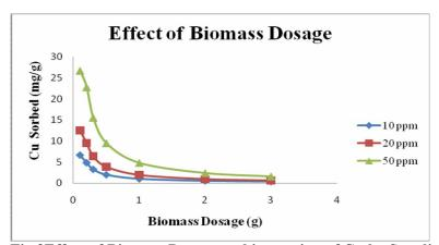
Fig.3Effect of Biomass Dosage on biosorption of Cu by Sprulina sp.(pH=5, initial Cu ion concentration = 10, 20 and 50 mg  $\Gamma^{-1}$ ; temperature = 25 °C; agitation speed = 120 rpm; contact time = 120 min).
