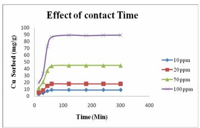
Fig.2 Effect of Contact Time on biosorption of Cu by Sprulina sp.(biomass dose=0.1 g, pH=5, initial Cu ion concentration = 10, 20 50 and 100 mg  $\Gamma^{-1}$ ; temperature = 25 °C; agitation speed = 120 rpm).
