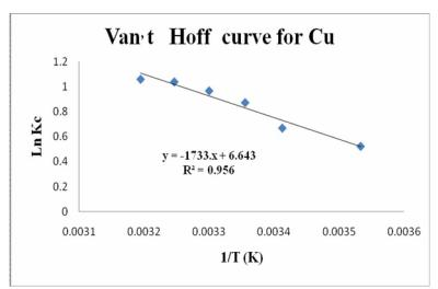
Fig. 8 Plot of Van't Hoff equation for the estimation of thermodynamic parameters for biosorption of Cu by Sprulina sp.
