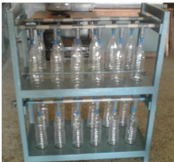
Fig 2: Algae bioreactor before experimentation
