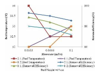
Fig 1 (b): Effect of Temperature on biofilter for the bed height of 65 cm
