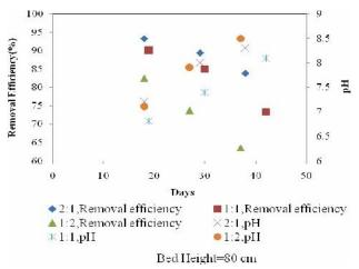
Fig 3 (c): Effect of pH on Biofilter for the bed height of 80 cm
