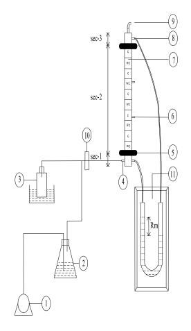
Gas temperatures before and after each column, bed temperatures, and ambient air temperatures were monitored with thermocouples and a temperature indicator system. Type-T (copper-constantant) thermocouples with welded and silicone coated ends were inserted into the centre of the reactor cylinders at locations previously displayed.
