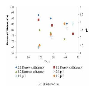
Fig 3(b) : Effect of pH on Biofilter for the bed height of 65cm
