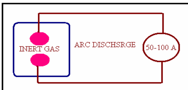
Fig.3. Diagrammatical representation of Arc Discharge setup for Synthesis and growth of nanotube
