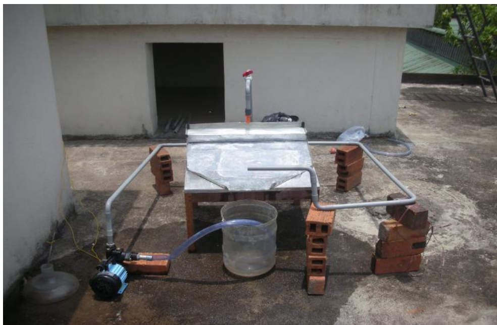
Fig 1 : Solar Trickle down flat plate reactor
