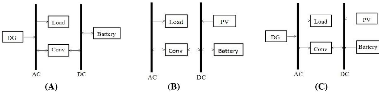
**Figure 1.** The schematic of the various system architectures, (A) Architecture - I (DG-BAT system), (B) Architecture - II (PV-BAT system), (C) Architecture - III (PV-DG-BAT).
