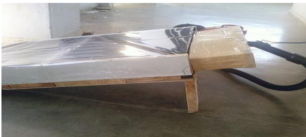
Fig. 2.2 Actual Experimental Setup of Double pass Solar Air Heater
