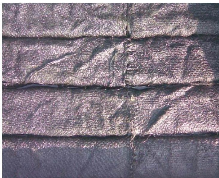
Fig.2 Porous absorbers of blackened jute fabric
