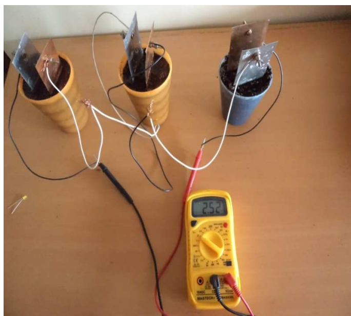
Plate 2: Three vermicompost cells in series produce 2.52V
