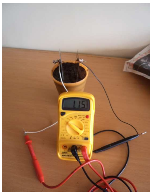
Plate 1: Single vermicompost cell produce 1.15V
