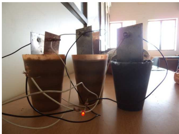
Plate 3: Vermicompost cell light up LED
