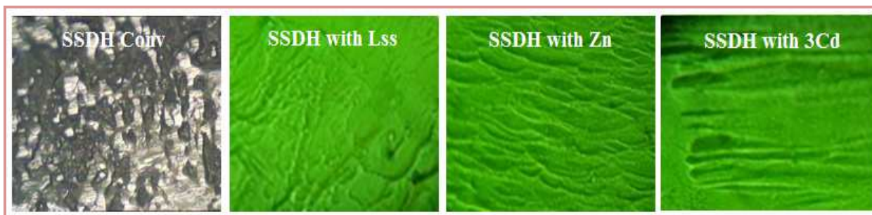
Figure 1.13(c) 15 sec, Etched surfaces of pure and doped SSDH crystal
