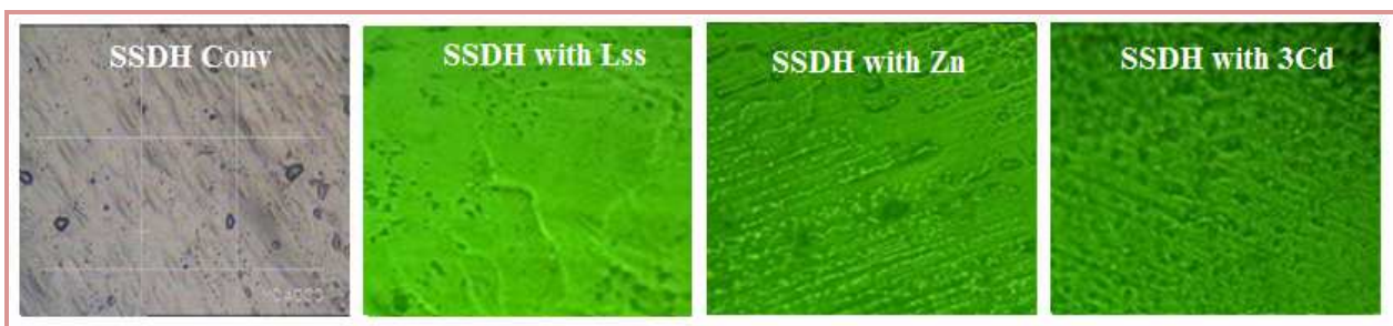
Figure 1.13(a) As grown surface of pure and doped SSDH crystal
