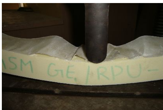
Fig.1: Buckling delaminations on the compressive face
