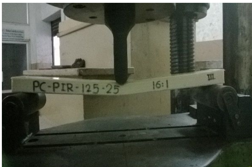
Figure 2. Three point bending test in a UTM for 21:1 span to depth ratio
