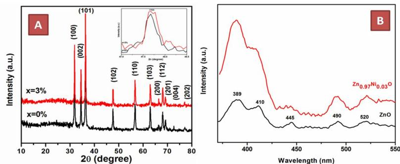
**Figure 1. (A) XRD patterns of  $Zn_{1-x}Ni_xO$  (0.0 and 0.03) samples. Inset shows the magnified area of (102) peak, (B) PL spectra of  $Zn_{1-x}Ni_xO$  (0.0 and 0.03).**
