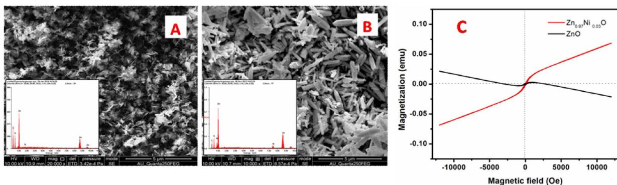
**Figure 2. SEM with EDAX images of (A) pure ZnO and (B) 3% Ni doped ZnO nanorods and (C) Magnetic behavior of (A) ZnO (B)  $Zn_{0.97}Ni_{0.03}O$  nanorods.**
