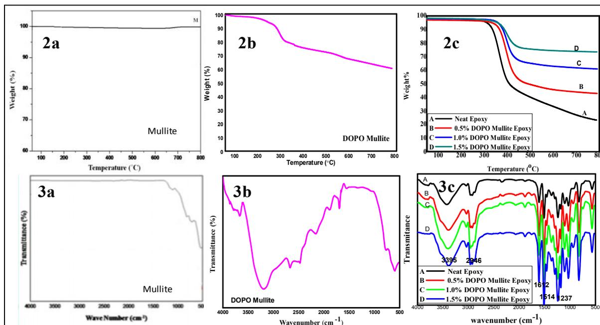
Figure 2: TGA of (2a) Mullite (2b) DOPO Mullite (2c) Neat, 0.5, 1.0, 1.5 wt % DOPO Mullite reinforced epoxy nanocomposites. Figure 3: FT-IR of (3a) Mullite (3b) DOPO Mullite (3c) Neat, 0.5, 1.0, 1.5 wt % DOPO Mullite reinforced epoxy nanocomposites.
