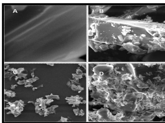
Figure 4 and 5: DSC & SEM image of (a) neat epoxy (b) 0.5wt % DOPO-Mullite (c) 1.0wt% DOPO-Mullite and (d) 1.5wt% DOPO-Mullite reinforced epoxy nanocomposites
