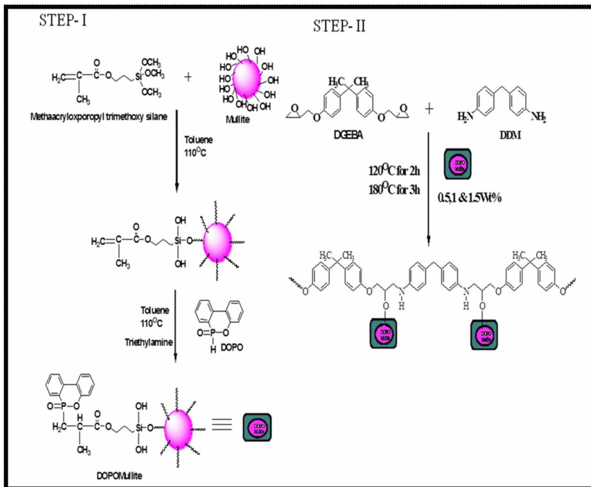
Figure 1: DOPO functionalized mullite fibre reinforced epoxy nanocomposites
