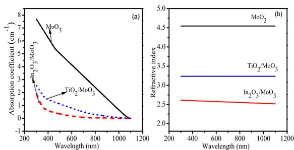
**Fig. 2** (a) Absorption and (b) Refractive index of  $\text{MoO}_3$ ,  $\text{In}_2\text{O}_3/\text{MoO}_3$  and  $\text{TiO}_2/\text{MoO}_3$
