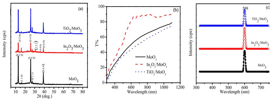
**Fig. 1** (a) XRD patterns (b) Transmission spectra (c) PL spectra of  $\text{MoO}_3$ ,  $\text{In}_2\text{O}_3/\text{MoO}_3$  and  $\text{TiO}_2/\text{MoO}_3$
