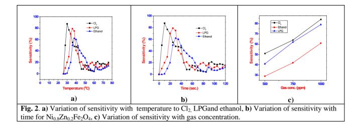
The variation of sensitivity with time is presented in Fig.2 b). The figure shows that, response increases with increase in time and then decreases. The sensor shows highest sensitivity at 11 sec to  $Cl_2$ . The variation sensitivity of the sensor with gas concentration is presented in Fig.2 c). It shows that the sensitivity of the sensor under investigation is lower at lower gas concentration and increases for increased concentration.
