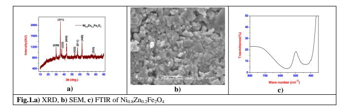
The infrared spectrum of  $Ni_{0.8}Zn_{0.2}Fe_2O_4$  is presented in Fig.1 c). It shows two major absorption bands near about 400cm<sup>-1</sup> and 600cm<sup>-1</sup> for octahedral and tetrahedral sites respectively. The lattice constant, crystallite size, grain size, absorption band and sensitivity are presented in the Table 1.
