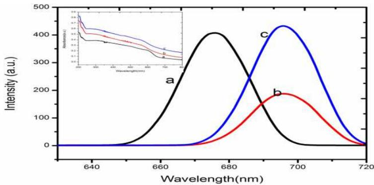
Fig. 4. UV-vis spectra and Photoluminescence spectra of (a) pure, (b ,c) CdSe:Cu nanocrystal.
