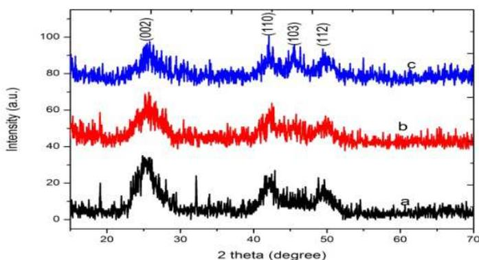
Fig. 1. XRD patterns of (a) CdSe, (b,c) CdSe:Cu nanoparticles.
