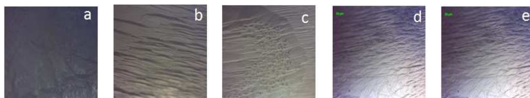
Fig 2. Surface of as grown TZNN single crystal a) without etchant, b) etching with water for 30sec, c) 45 sec, d) 1 min, e) 2 min [20 x magnification]
