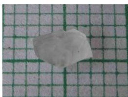
Fig 1. Photograph of as grown GLS single crystal
