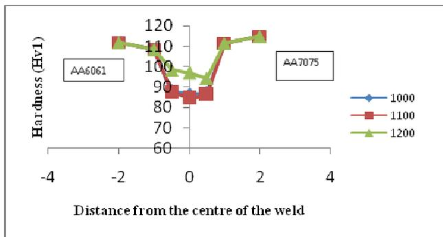
Fig 2 :Microhardness at different tool rotational speeds
