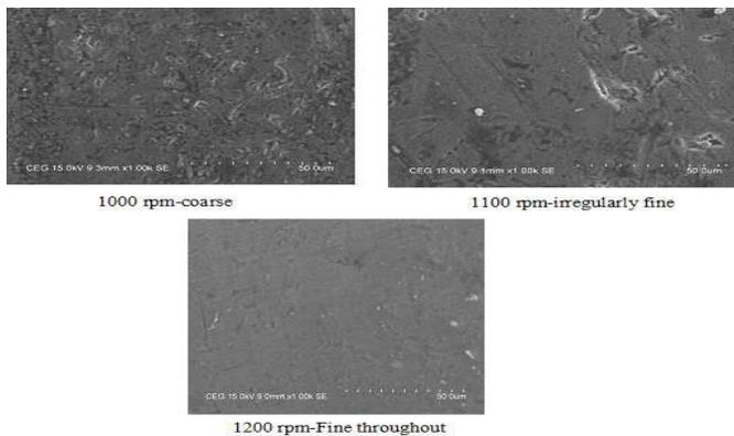
Fig 3: 1000X SEM micrographs for different tool rotational speeds
