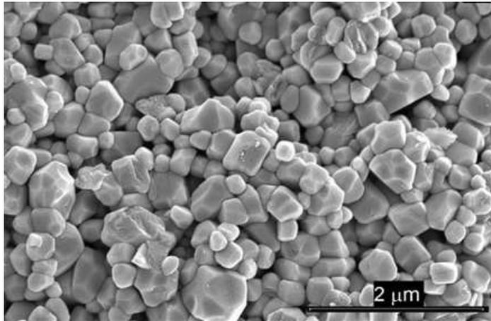
Fig.1: HRSEM of fractured surface of sample after HIP.
