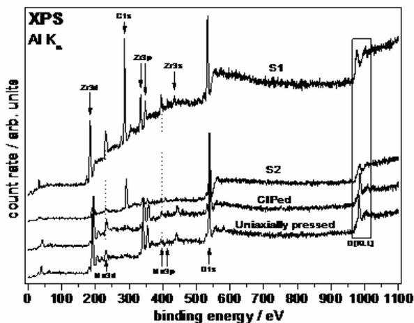
Fig. 2: XPS spectra of the uniaxially pressed, CIPed and HIPed samples (S1 and S2).
