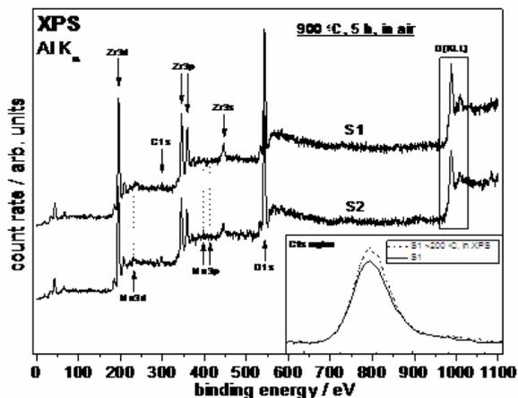
Fig. 3: XPS spectra of samples S1 and S2 after heating in air at 900 °C (5 h). Inset: The C (1s) level of sample S1 heated up to ~ 200 °C inside the XPS apparatus.
