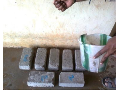
Fig. 11 Curing of Bricks
