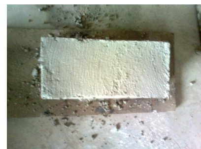
Fig. 9 Casted Brick Kept for Air Curing
