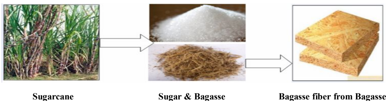
Fig. 2 Formation of Bagasse Biocomposite material
