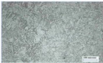
Fig. 7: The interfaces of SAW weld metal at 170 X
