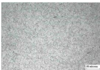
Fig .3: Micrograph of the face side weld metal (SAW) at 170X
