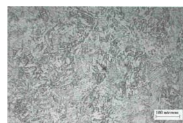
Fig.4: Micrograph of the weld metal (SAW) 2 mm from the top at 170X
