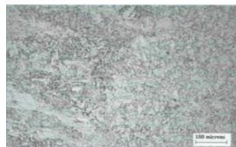
Fig.8: The interface SMAW weld metal at 170 X
