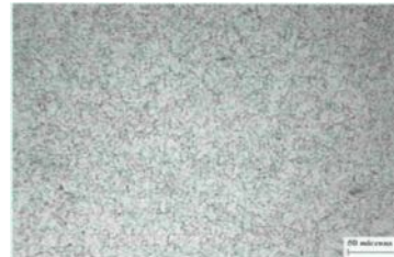
Fig .1: Micrograph of the P91 base metal at 340 X Fig.2:Micrograph of HAZ at 340 X
