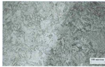
Fig.6: The interface between GTAW & SMAW WM at 170 X
