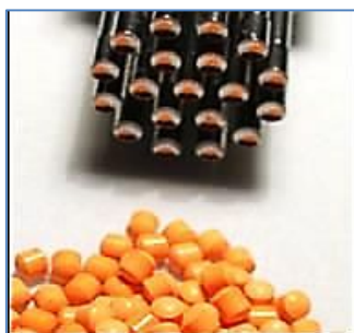
Fig No 3: Compressed and coated mini tablets
