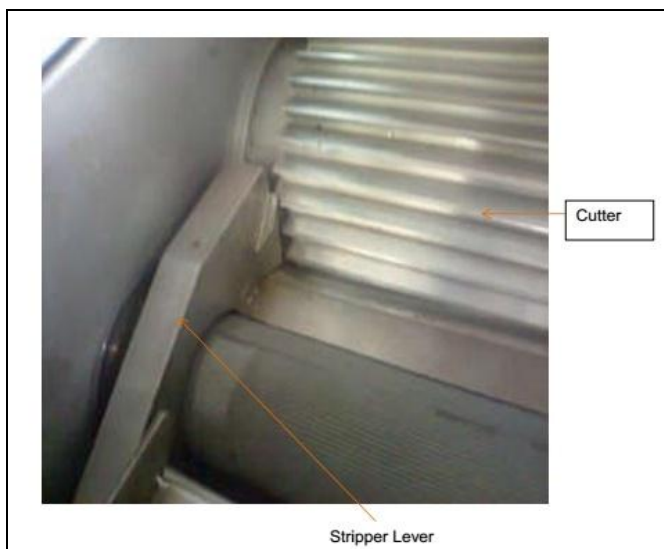
Fig. 13: Modified lever plate
