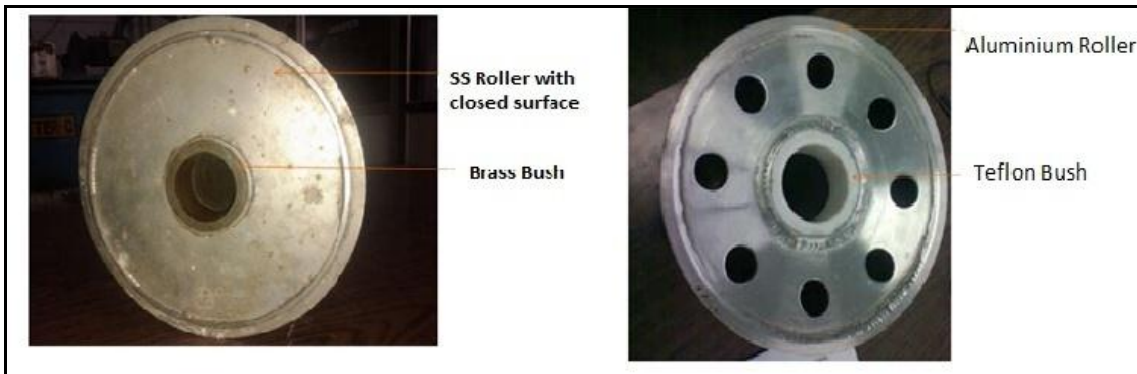
Fig 8: SS 304 roller with closed surface
