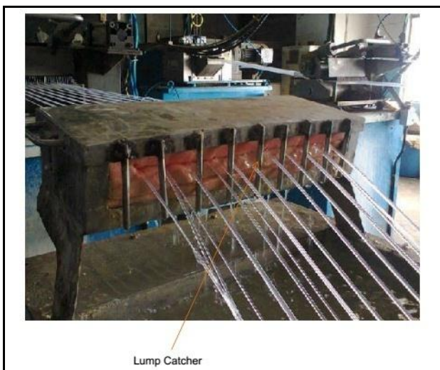
Fig 10: Joint strand / lump catcher
