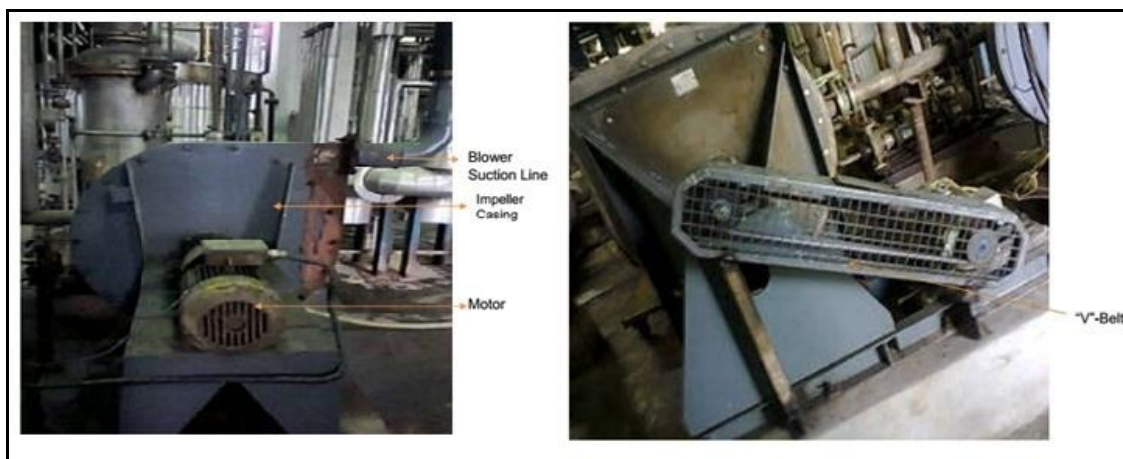
Fig 6: Direct Driven MS Body/ Impeller monomer suction blower
