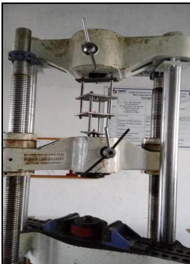
Fig. 5 Universal Testing Machine clamped with Miniature Specimen
