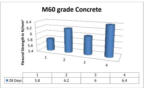
The Flexural strength of conventional concrete and modified concrete i.e with the replacement of Fine Aggregate with M –Sand at the age 7 and 28 days of Flexural Strength with adding the Super Plasticizers 0, 1, 1.3 respectively. The Flexural strength is increase as the percentages of M – Sand increases with 1.3% of SP 100 when compares to 1% of Super plasticizers.
