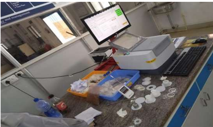
Fig 6: The XRF Photospectrometer for evaluating the nonmetals/ions/metals and REE's
