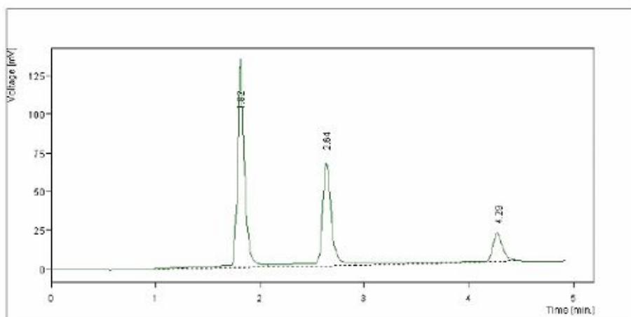
Figure 1. Standard Chromatogram of Paracetamol, Chlorzoxazone and Aceclofenac
