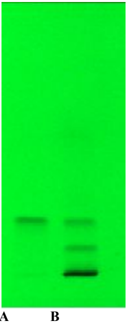
Figure 1: Photograph of chromatograms obtained, at 380 nm, from quercetin standard (A) and a hydroalcoholic extract (B) of the dried flower of N. stellata Wild.
