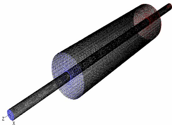
**Fig 1 Grid for membrane reactor**
