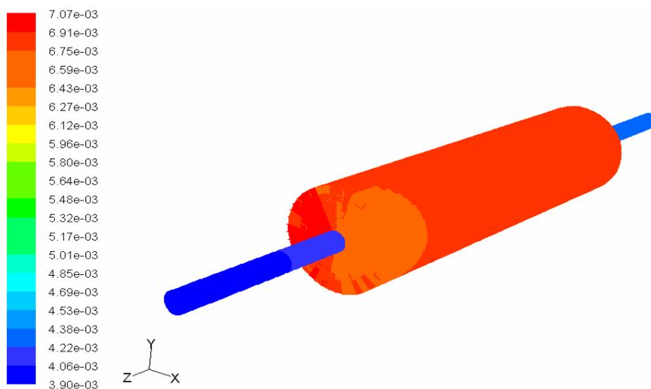
Fig 2  $H_2$  contour for time factor 4140 g min/CO mol, 595 K, sweep flow rate of 436 ml/min,
