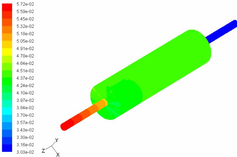
**Fig 3** H<sub>2</sub> contour for time factor 4140 g min/CO mol, 595 K, sweep flow rate of 436 ml/min, lumen pressure of 2.5 atm, shell pressure of 1 atm and steam to CO ratio of 2.5
