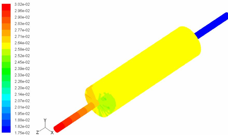
**Fig 4** H<sub>2</sub> contour for time factor 4140 g min/CO mol, 595 K, sweep flow rate of 436 ml/min, lumen pressure of 2 atm, shell pressure of 1 atm and steam to CO ratio of 2.5
