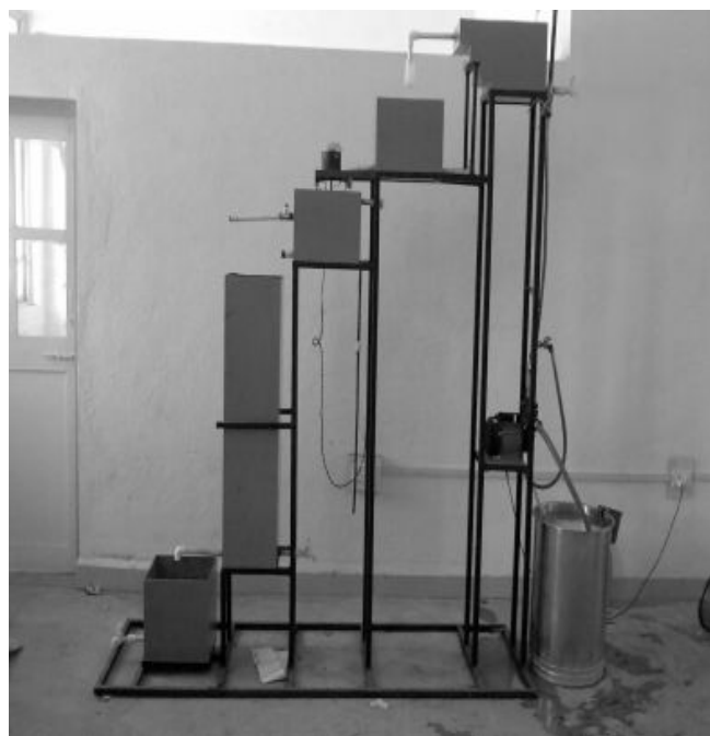
Fig.1. Laboratory scale grey water treatment system
