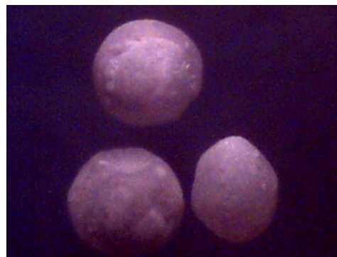
Fig. 2: Photomicrograph of ethyl cellulose coated microcapsules, Magnification 200x.
